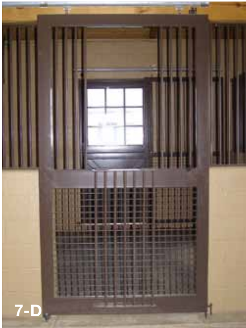
7-D Wide-frame steel sliding door with steel bars on top and fold-down straight yoke. Crosshatch mesh bottom. 6-inch steel center rail and 6-inch bedding guard.
